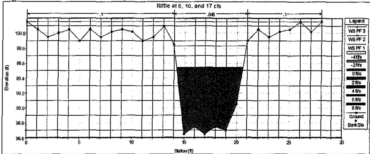
Hydraulics results for the riffle cross-sections show velocities of 1.34 ft/s and 1.47 ft/sec at 6 cfs and 17 cfs respectively (Tables 2 and 3). Shear stress values were 0.12 lbs/ft<sup>2</sup> and 0.20 lbs/ft<sup>2</sup> at these same flows.
